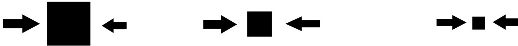
Figure 1.1: A cube made of auxetic material shrinks in all directions when squeezed in only one direction.
