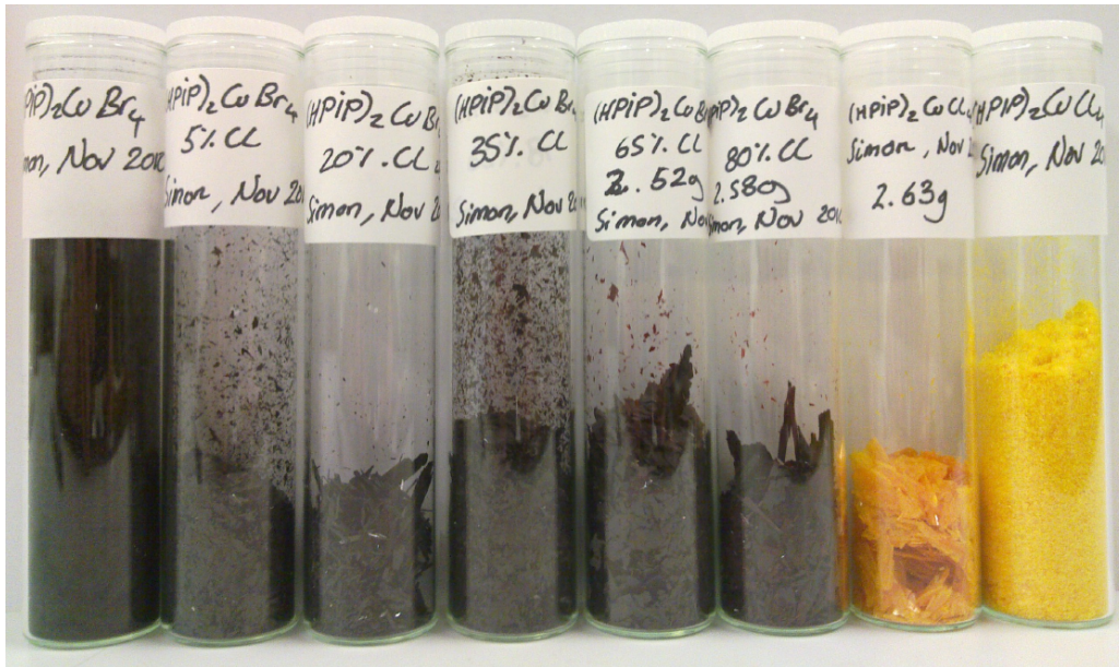
Fig. 1.2: Bromine doped BPCC is shown. The black probe on the left contains only bromine atoms and the one on the right only chlorine atoms. The probes in between contain both sorts and the concentration of chlorine is increased from left to right. The picture is taken from the PhD thesis of Simon Ward who investigated the properties of these doped materials by neutron scattering measurements [13].
