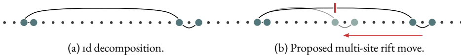
Figure 3.9: (a) Only moving single sites around leads to a decomposition of the graph. (b) To counter this, a new multi-site rift move is introduced which chooses a random site, divides the graph into two subgraphs and moves one of the clusters by a random length.
