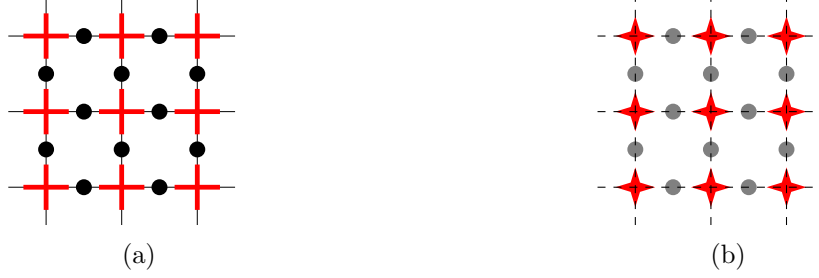
Figure 2.7: (a) The toric code on the square lattice with marked stars. (b) Dual lattice where the stars are lattice sites of again a square lattice, while original spin-sites lie on the bonds.
