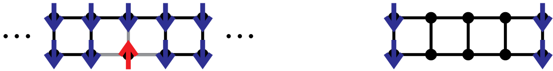
Figure 29: Left: State with one spin-flip. The corresponding excited bonds are marked in grey. Right: Cluster with a fixed environment. Such a cluster is used, to calculate the hopping terms of the one spin-flip.
