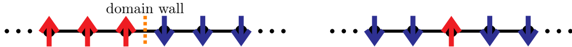
Figure 15: Left: domain wall as fundamental excitation in low-field limit. Right: spin flip as fundamental excitation
